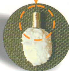
3.5ml cement injected into the size 20 of Vessel-X ®
